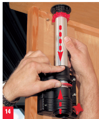
14. Push the automatic clamp plate up and insert the mast. Place the mast vertically so that it is easy to move it.
