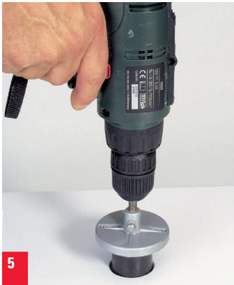
5. Use the circular drill bit to drill a hole from the roof.
